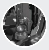
**K80 ball-head coupling**Ideal for heavy-duty trailer operation.
