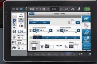
The new pressurized HVAC climate control system features more vents and louvers to increase air flow around the operator. It can also be controlled directly via the encoder or the configurable buttons.
