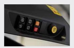
**Easy to reach** External controls on both fenders for easy implement connection.
