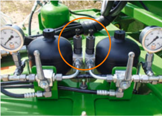
Drawbar damping system as standard
