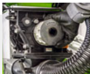
Easy exchange of the metering rollers
