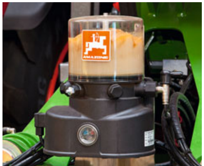
Pump with reservoir
