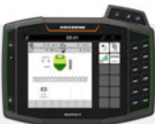
Convenient operation via the ISOBUS terminal
