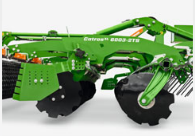
Catros XL 6003-2TS at its deepest working depth – the discs are completely swivelled away from the frame
