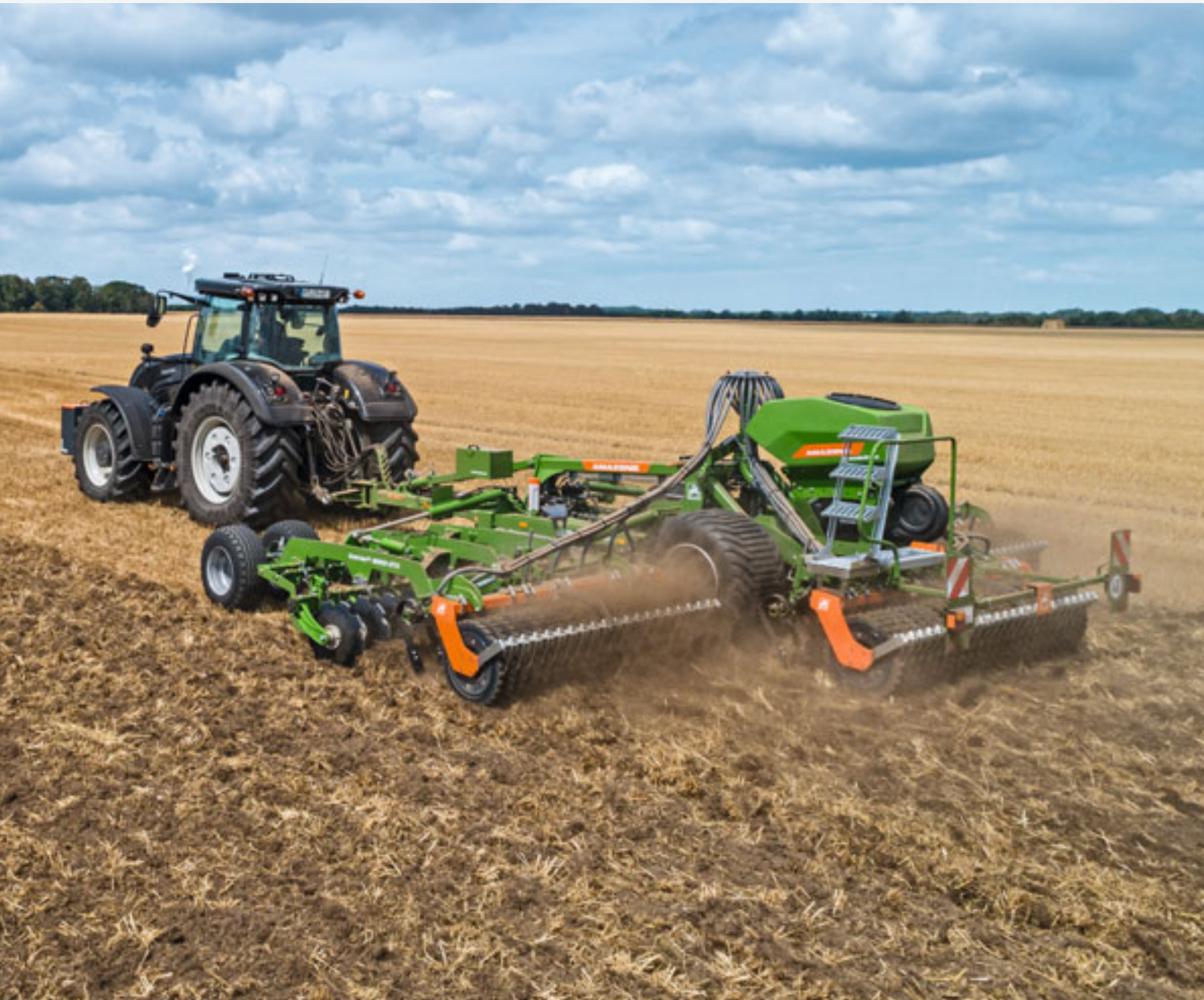
Catros XL 8003-2TX with wedge ring roller with Matrix tyre profile in 8 m working width
