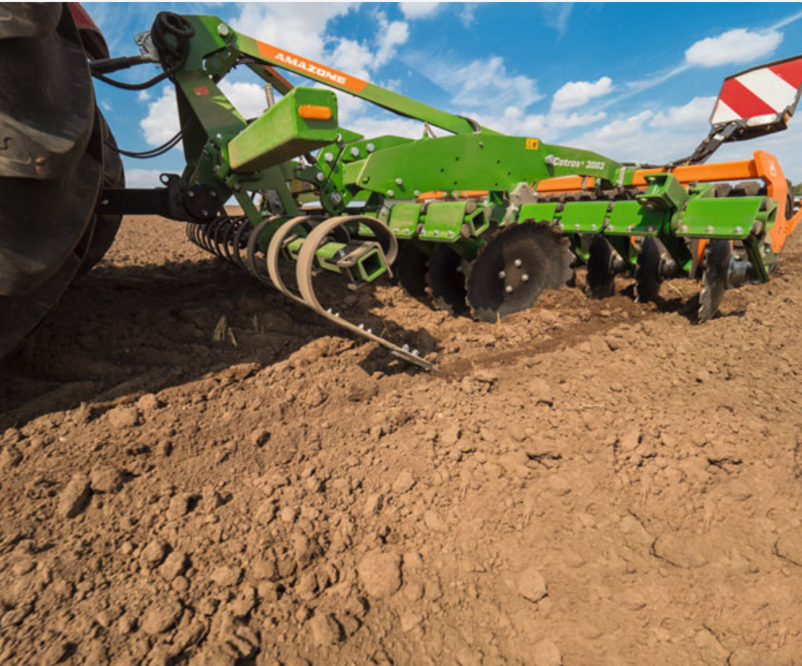
Catros+ 3003 in operation with the Crushboard
