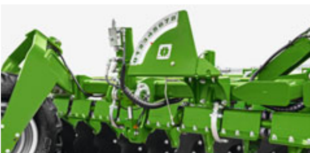
Hydraulic working depth adjustment with easy-to-read scale
