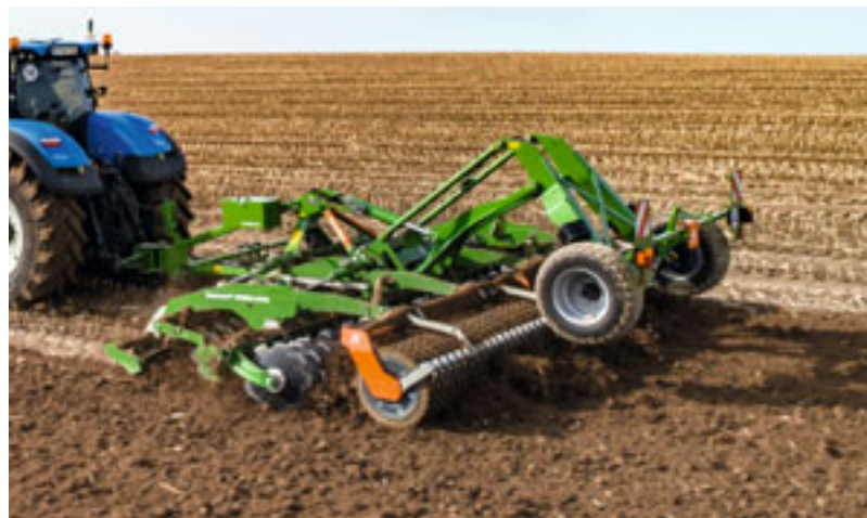
Catros XL 6003-2TS with up-front knife roller
