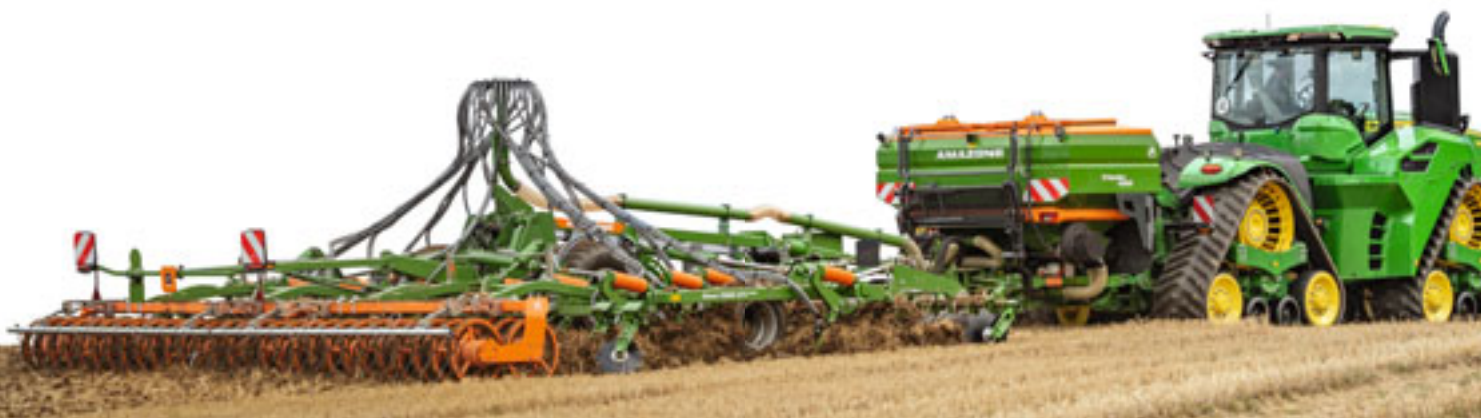
XTender 4200 mounted hopper with a capacity of 4,200 l with Ceus 7000-2TX
