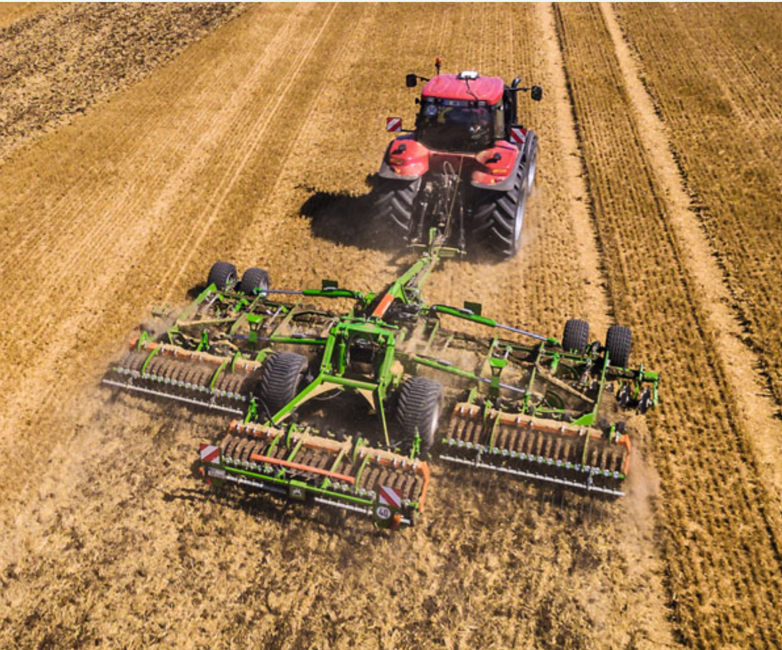
Catros + 8003-2TX with wedge ring roller with Matrix tyre profile in 8 m working width
