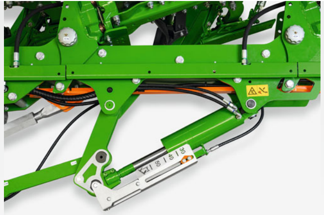
Hydraulic adjustment of the furrow width
