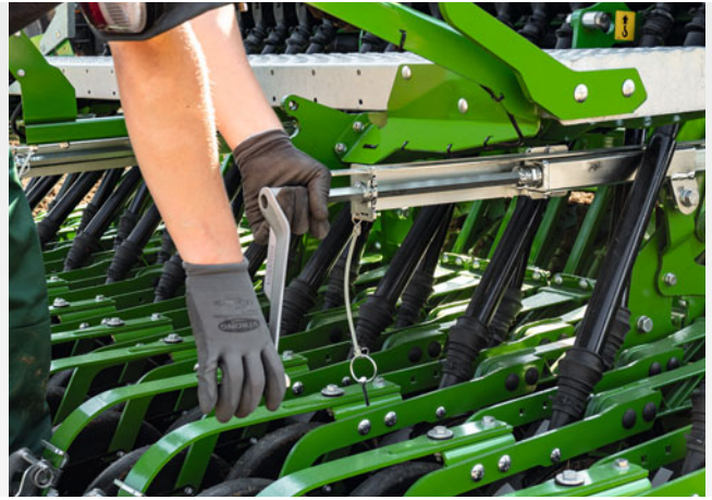
Simple setting of the placement depth on the right and left sides from around the back of the Cataya Special
