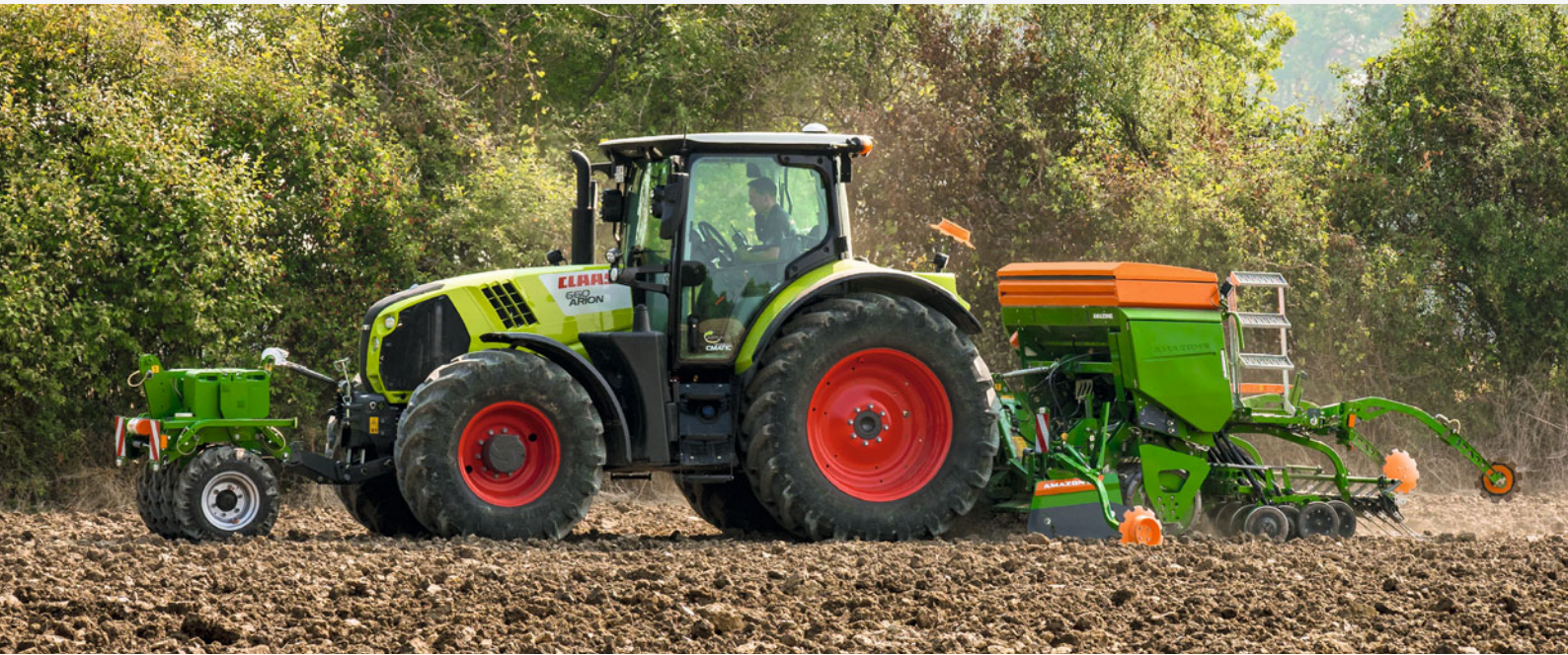
Cataya 3000 Super with T-Pack U front tyre packer sowing after the plough
