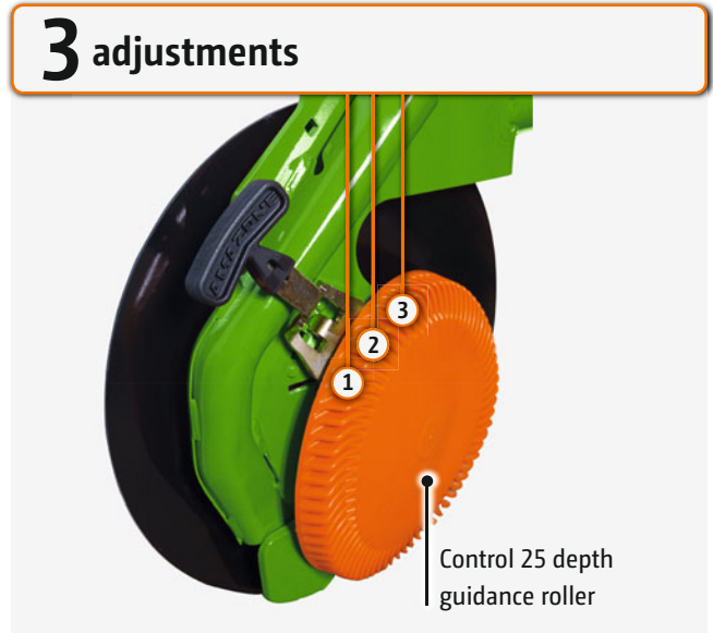
✓ RoTeC coulters (Ø 320 mm) with Control 25 depth guidance roller
