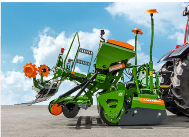
Hydraulic coulters lift of the Cataya Special
