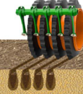
KWM wedge ring roller with Matrix tyre profile/600 mm
