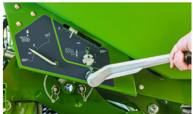
Central, infinitely-variable mechanical coulters pressure adjustment with setting scale on Cataya Super
