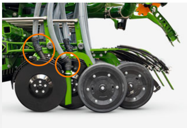
TwinTeC couler with an additional outlet
