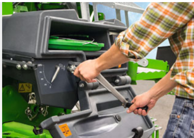
Central setting of the sowing depth
