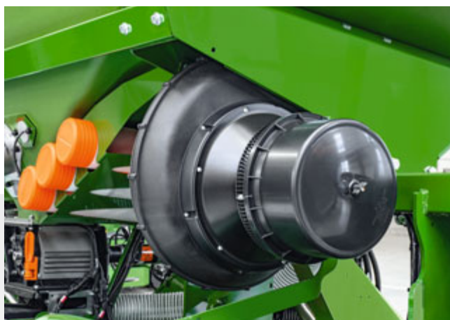
The optional cyclone separator reduces the dust load
