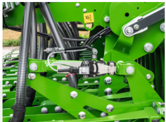
Cylinder for the hydraulic coulters pressure adjustment
