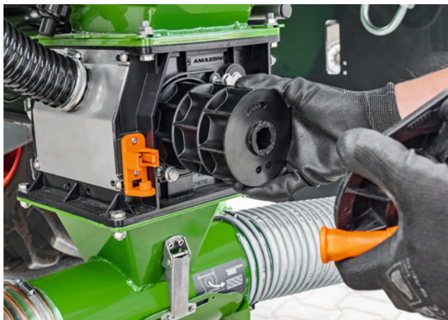
Simple exchange of the metering rollers on the FTender
