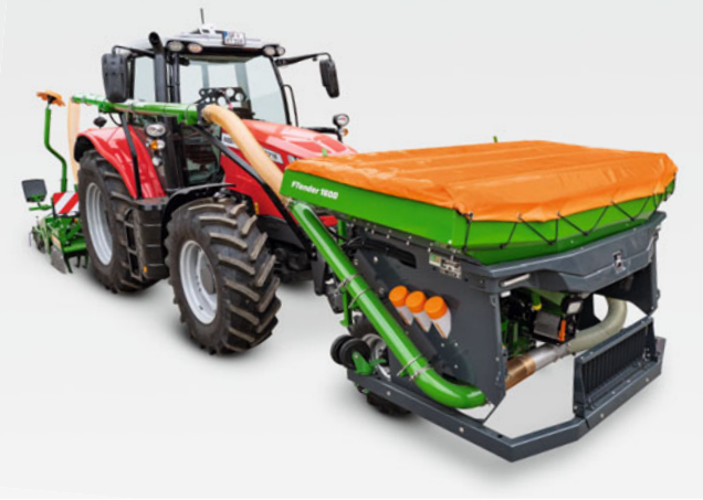
FTender 1600 with open conveyor system with roll-over tarpaulin
