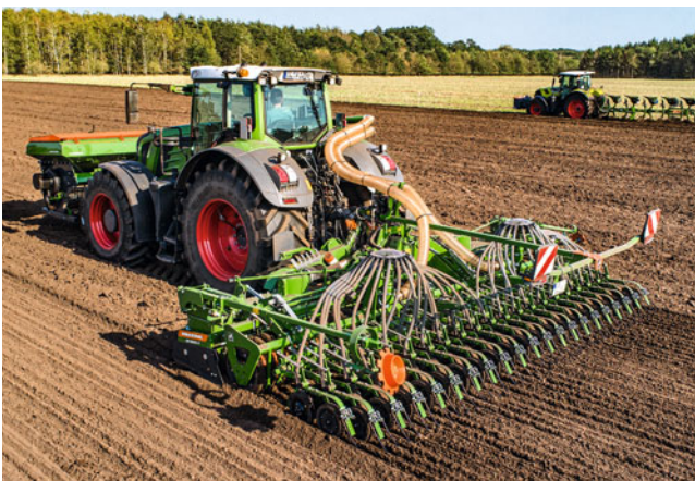
Folding KG 6002-2 in 6 m working width and mounted Avant seed rail with TwinTeC coulters
