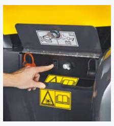
Hood raise switch, battery kill switch and remote battery terminals are grouped at the rear
