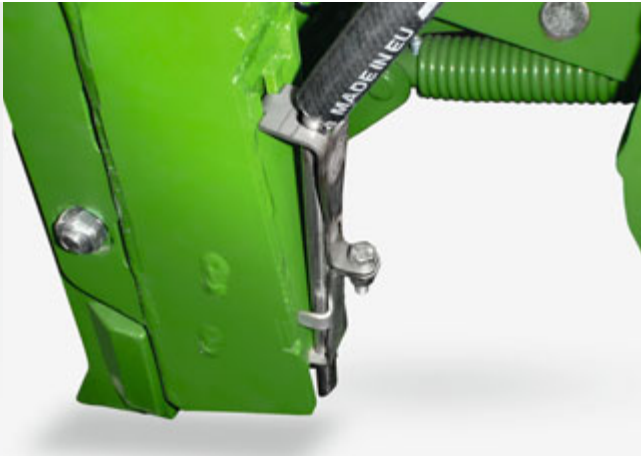
Neat routing of the fertiliser hoses to the outlet on the chisel openers of the Primera DMC
