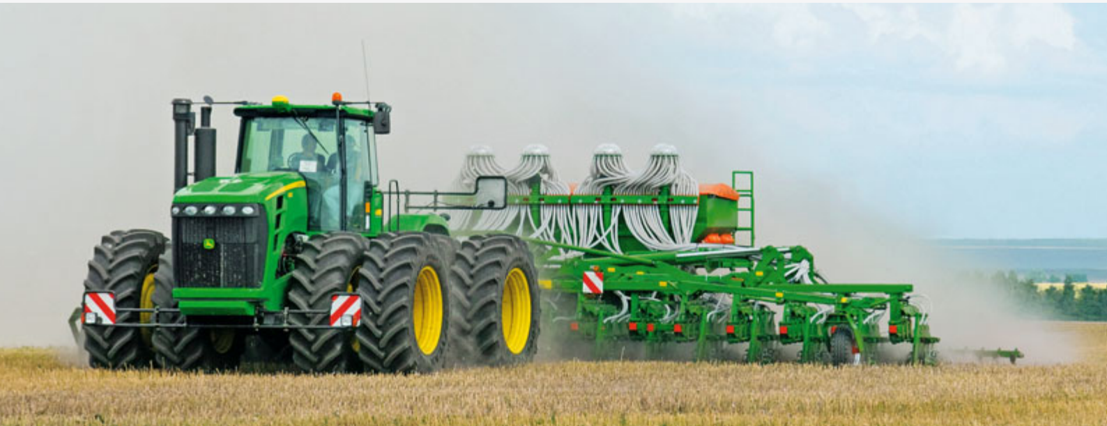
Primera DMC 12000-2C, 12 m working width
