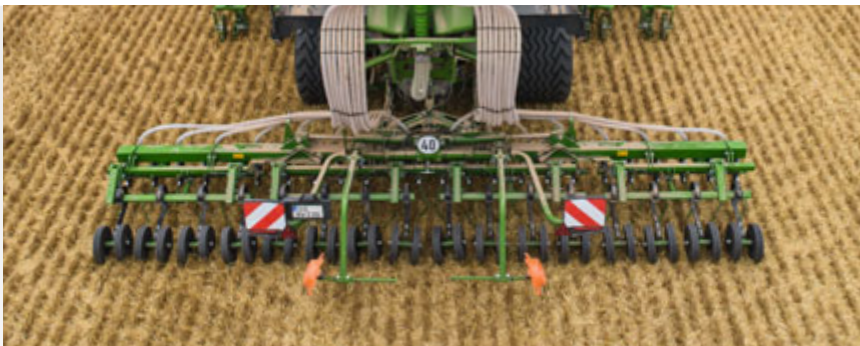
Pre-emergence markers for the Primera DMC 6000-2C
