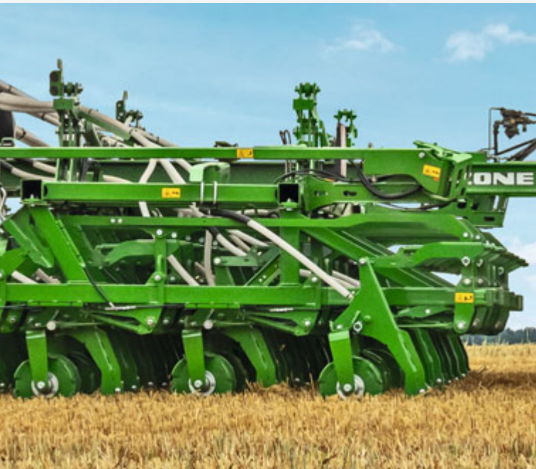
Parallelogram suspension of the chisel openers
